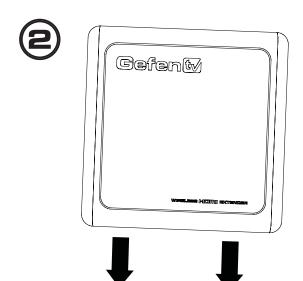
To place a main unit into a stand, first orient the front of the stand (where the logo is located) with the LED's on the front panel of the main unit. Lower the unit into the stand. There are channels (a) located on both the main unit and stand that will help guide the main unit into the stand.
